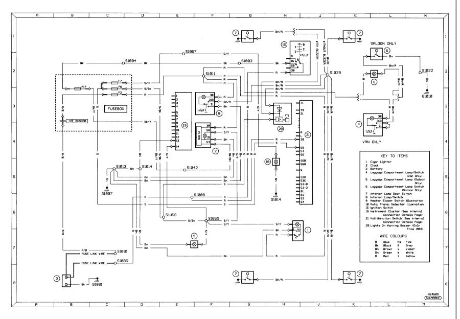
Diagram 2b: Interior lighting, lights-on warning buzzer, clock and cigar lighter
